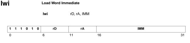
Loads a word (32 bits) from the word aligned memory location that results from adding the contents of register rA and the value IMM, sign-extended to 32 bits. The data is placed in register rD.
